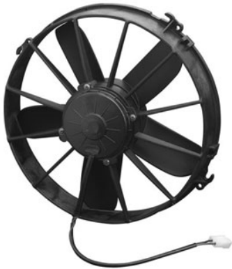
30102025 Weight: 5.25 lbs 12" Paddle Blade High Performance Fan / 12V Pusher for AC condensers 2780m 3 /h. 16.5A
