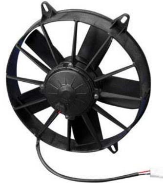
30102040 Weight: 5.5 lbs. 11" Paddle Blade High Performance Fan/ 12V Pusher for AC condensers. 2310m 3 /h. 14.0A
