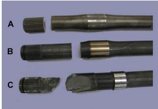
A KAM Aerospace 9403 Nm B KAM HD 7132 Nm C Land Rover 4800 Nm
